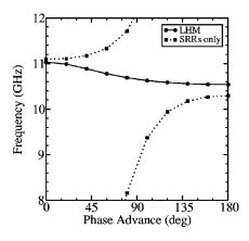
FIG. 2. Numerically simulated dispersion curves for the LHM and "SRR only" material. Notice that the solid curve has a negative slope  $(d\omega/dk < 0)$ . The lower, dotted curve continues to zero frequency at zero-phase advance.
