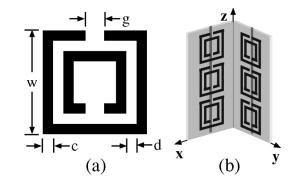
FIG. 1. (a) Diagram of a single split-ring resonator (SRR), c = 0.25 mm, d = 0.30 mm, g = 0.46 mm, w = 2.62 mm, and the SRR is square. (b) Each unit cell has six copper SRRs and two wire strips on thin fiberglass boards. The wire strips are 1 cm long, centered on the SRRs, and on the opposite side of the board from the SRRs. The angle between the fiberglass boards is 90° to make square unit cells with a lattice constant of 5.0 mm.
