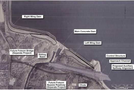
Figure 5. Potential Auxiliary Spillway
