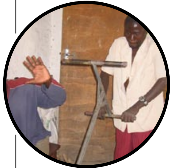
Operation of a ram press. (Mwape, Zambia 2005)
