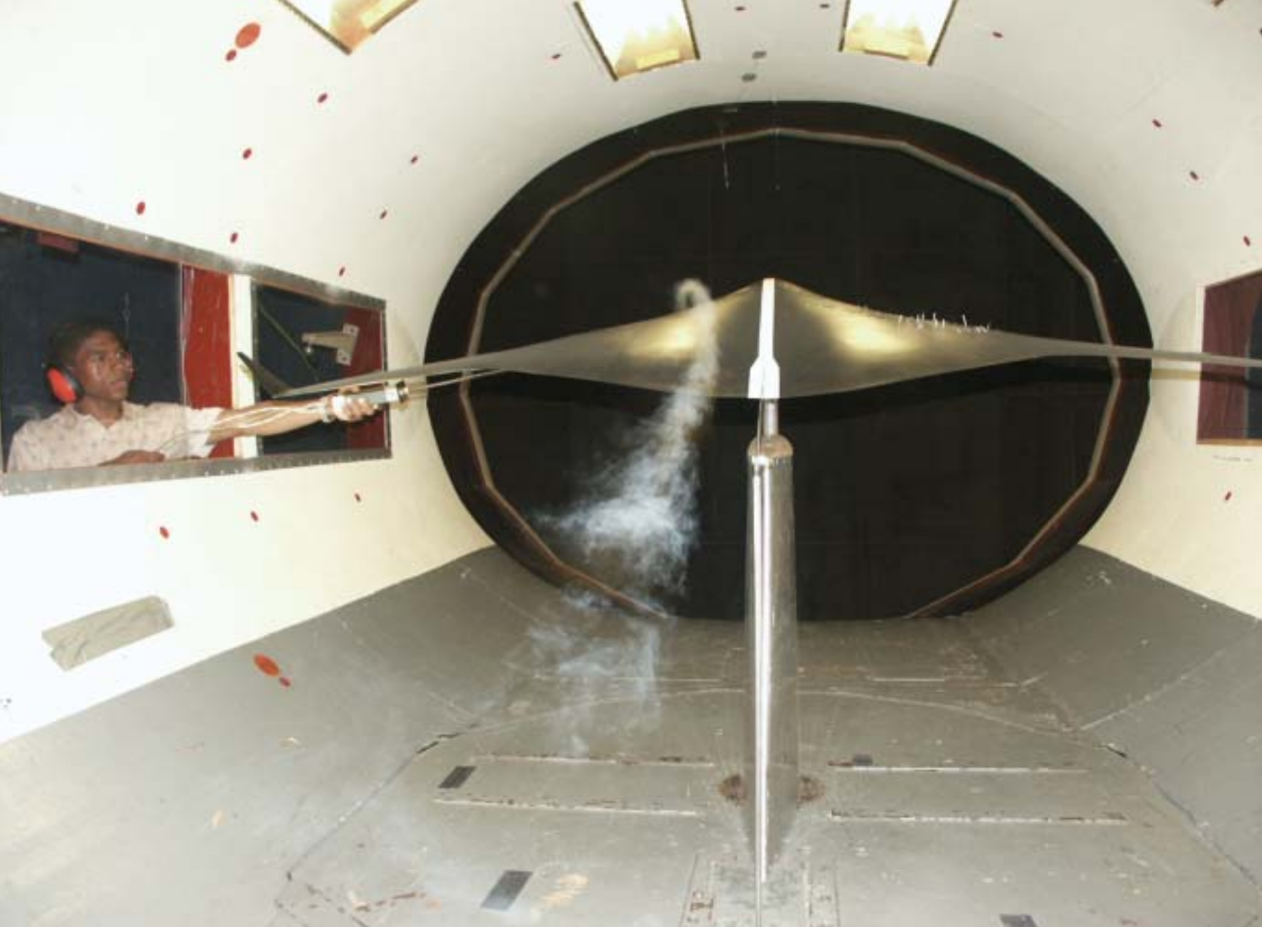
Aero-Astro senior Christopher J. Sequeira performs a flow visualization in the Wright Brothers Wind Tunnel to detect separated flow over a blended-wing body aircraft model. A project-based approach to learning, such as this, offers students an immediate opportunity to apply theory to problems approaching the complexity of modern aircraft. (William Litant photograph)
