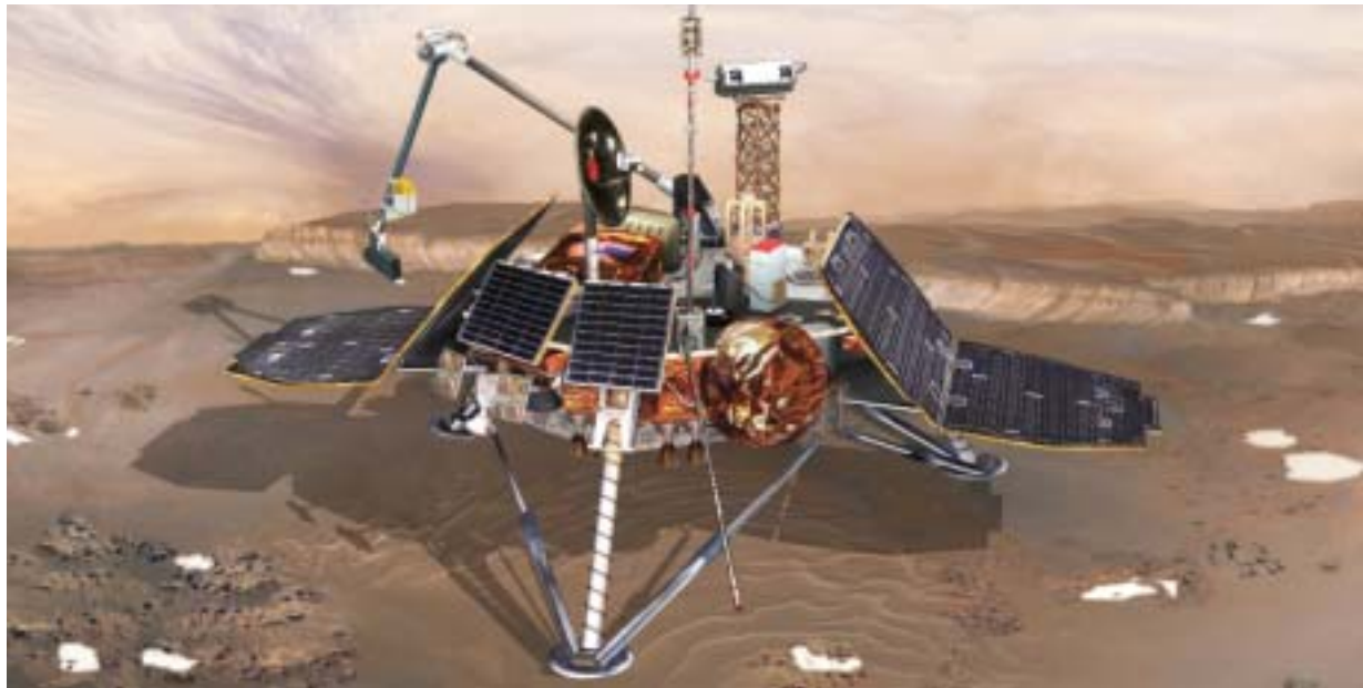
It's believed that the 1999 loss of the Mars Polar Lander was the result of software shutting down the landing engines while the craft was still 40 meters above the Martian surface. (NASA illustration)
