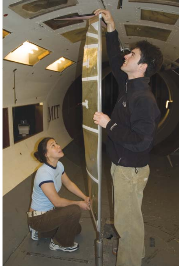
In the Wright Brothers Wind Tunnel, 16.62X students Sunny Wicks and Ben Stewart prepare to test a drag-reducing winglet they designed for the top of America’s Cup ship sails. (William Litant photograph)
