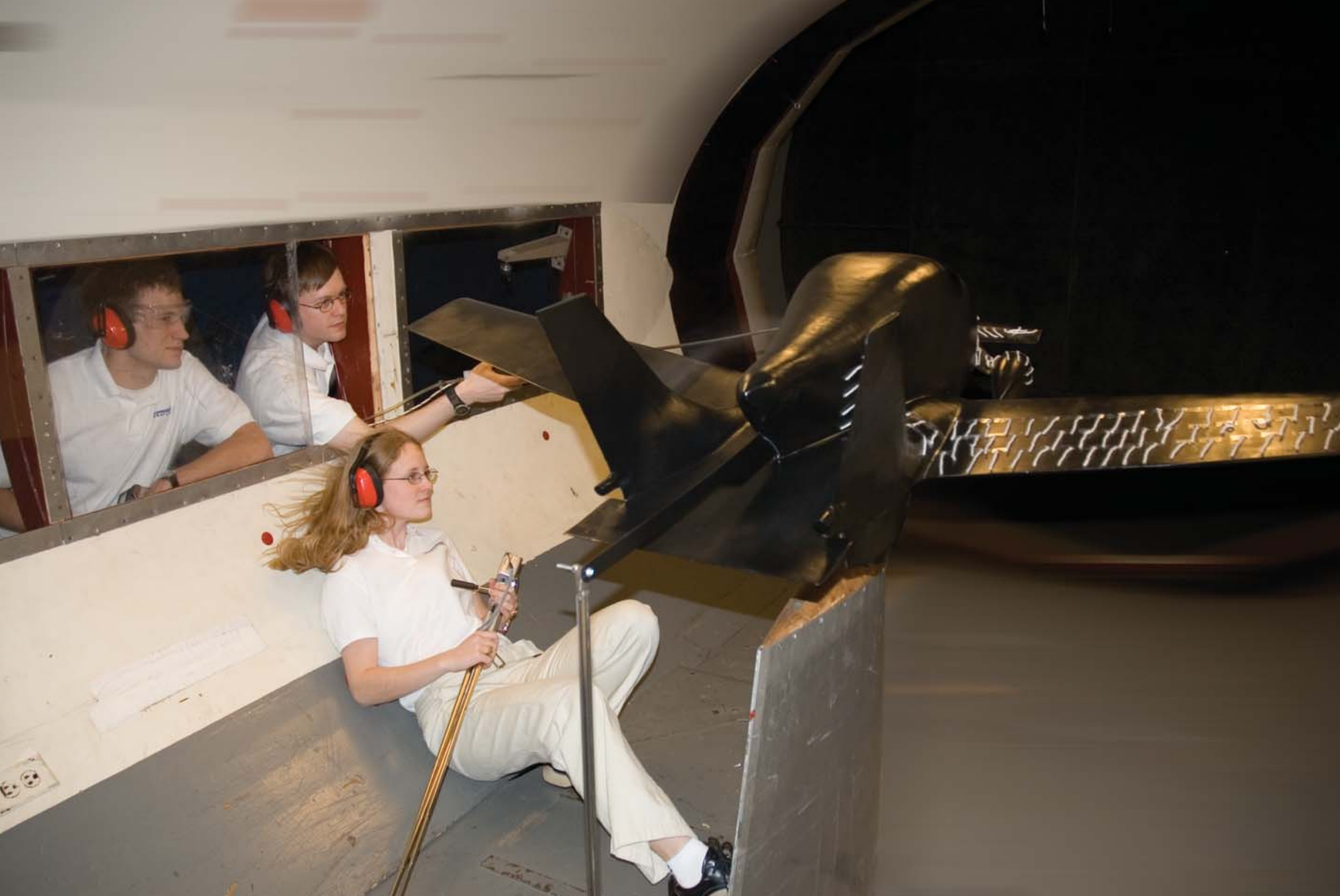
In Aero-Astro's Wright Brothers Wind Tunnel, graduate student Anna Mracek, recent alumnus Dr. Samuel Schweighart (left), and doctoral candidate Carl Dietrich run tests on a model of Transition, the roadable airplane they hope to manufacture. (William Litant photograph)
