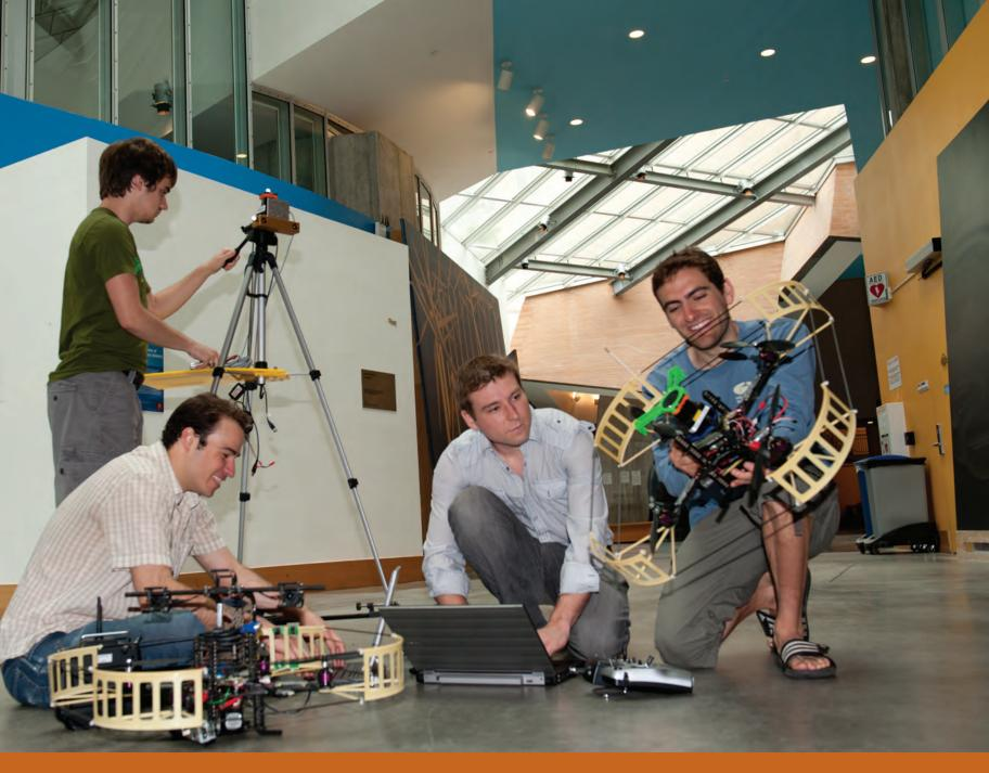
Students (from left) James Wiken (standing), Abraham Bachrach, Samuel Prentice, and Adam Bry prep a pair of quadrotor helicopters to fly through MIT's Stata Center, exploring and mapping the building. Equipped with a variety of sensors for operating in different environments, the rotorcraft can fly in complex, populated environments. (William Litant/MIT photo)
