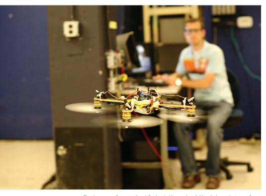
The Aerospace Computational Design Lab's novel variable-pitch quadrotor performs maneuvers beyond the capabilities of off-the-shelf fixed-pitch quadrotors, including flying upside down, as this one demonstrates. (Bernard "Buddy" Michini/MIT photo)
