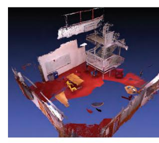
A 3D map of an MIT lab space multi-story environment generated using a Microsoft Kinect during an autonomous quadrotor flight. The Kinect was originally developed to enable interaction with the Xbox 360 by using gestures, obviating the need touch a controller.
