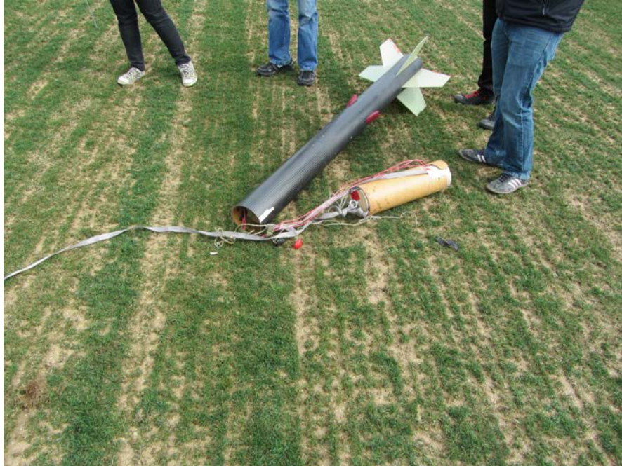
FIGURE 17: MAIN BODY AFTER LANDING WITH MAIN PARACHUTE INSIDE
