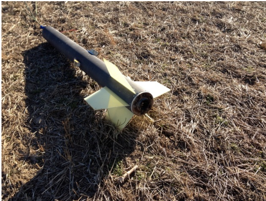
FIGURE 14: MAIN BODY AFTER LANDING WITH MISSING LIBERATED FIN
