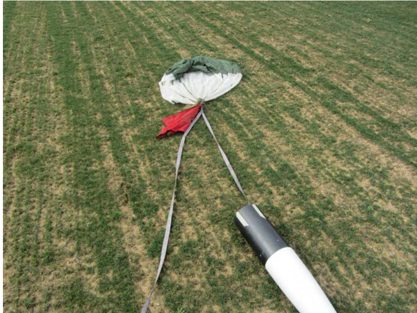
FIGURE 16: UPPER BODY WITH DROGUE PARACHUTE DEPLOYED
