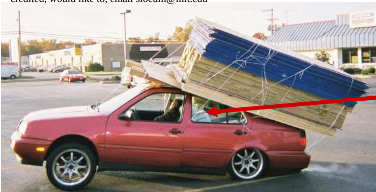
Ten 80 lb bags of concrete
