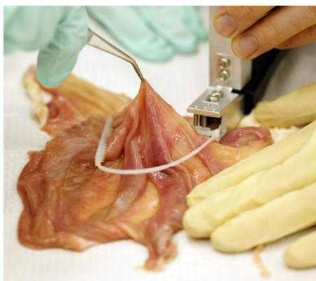
Fig. 16 A photograph of a first generation spiky clamp being closed onto sheep stomach tissue
