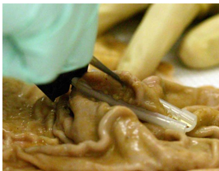
Fig. 10 Photograph of the final prototype beam deflection while clamping pig stomach tissue
