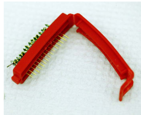
Fig. 4 An early prototype spiky clamp concept, consisting of a pair of beams, hinged at one end and with a snap-fit latch at the opposite end. A row of spikes is set in one beam to provide a piercing element.
