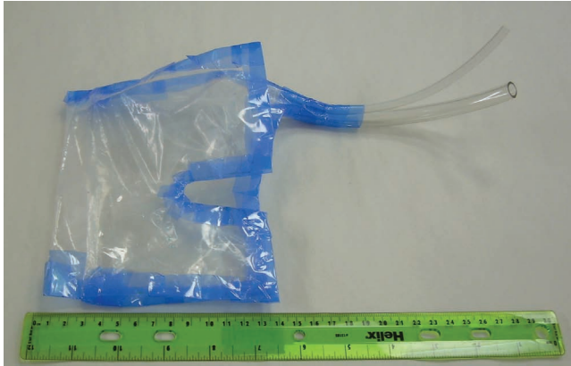
Figure 5. A mockup of the “taco shell” bag, an early predecessor to the final Kidney Cooler device.
