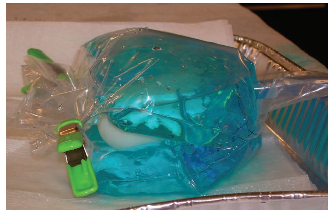
Figure 2. The final bag prototype wrapped around a model kidney and filled with fluid
