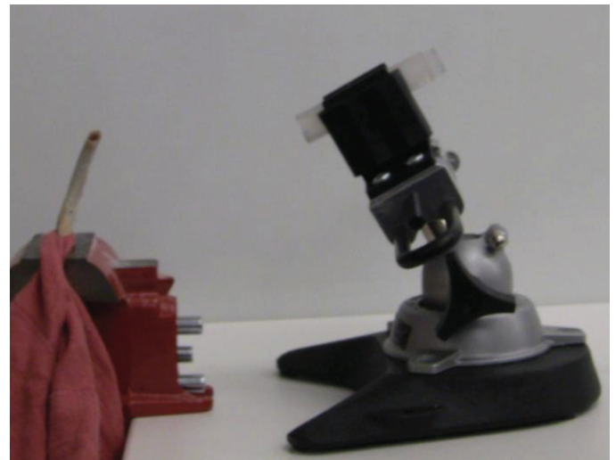
FIGURE 16 – MOCK SETUP, INCLUDING TROCAR SLEEVE AND RIB, USED TO TEST THE ENDOSCOPIC DRIVER PROTOTYPE. THE TROCAR SLEEVE IS SIMULATED BY A SIMPLE PLASTIC TUBE AND THE RIB IS FIXED IN A VICE.
