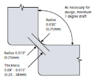
A slightly different hinge design is shown in Figure 3. Although not as efficient as the basic design shown in Figure 1 and with a more limited angular movement, this design will allow the hinge to be molded at an angle to the tool parting plane.
