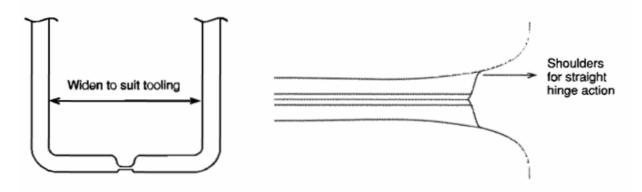
As shown in figure 2, the inclusion of shoulders allows for an increase in the thickness of the section of the mold where the hinge is to be formed, thus preventing any bowing or breaking of the steel insert.
