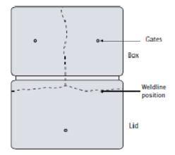
Fig. 12. Cating on both sides of hinge
