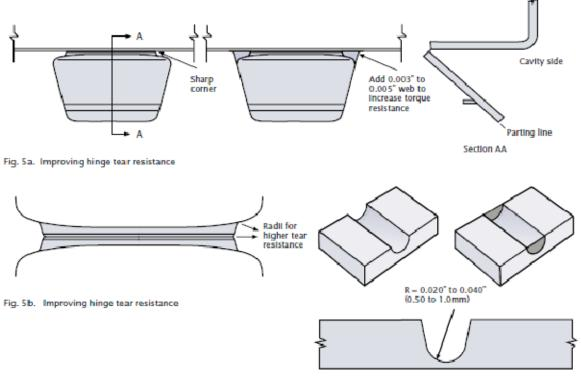
Fig. 6. Increasing tear resistance by adding thin web ends of the hinge
