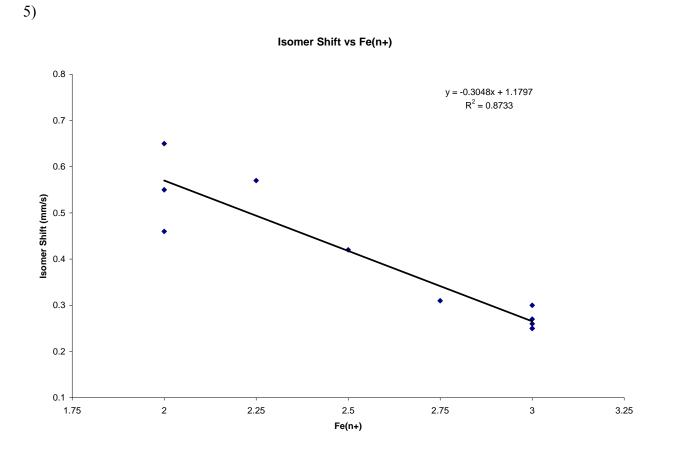
For Fe<sup>n+</sup>, given n = -0.3048\*(isomer shift) + 1.1797 and the observed isomer shift of 0.37 mm/s, the predicted iron valence from the fit is n = 2.66. This non-integral number for the valence of iron indicates that an averaging process is taking place to produce a mixed-valence species (i.e. six Fe<sup>2.66+</sup>). To get the formal oxidation states of the iron ions, we first multiply the
