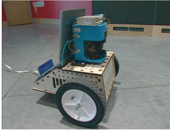
Figure 7: Splinter. This is the robot that collected the dataset. The vehicle, known as “Splinter”, has high quality quadrature phase encoders on each drive motor. A laptop on the back of the vehicle logged the data. The large blue device in the front of the vehicle is a laser range finder, not used in this article.
