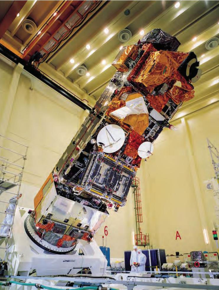
Launched in 2002, the European Space Agency's Envisat is the largest Earth observation satellite ever built. With 10 instruments and a mass of more than eight metric tons, it is expected to operate at least until 2013. This type of huge multi-instrument platform is of great use to scientists as it facilitates data cross-registration between instruments. However, multiple interferences among instruments made the development of this satellite an engineering nightmare. (NASA image)
