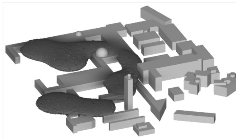
New computational methods are being developed to estimate physical properties from observational data. Here, the initial conditions of a contaminant release are estimated from synthetic measurements of contaminant concentration at sensor locations scattered throughout the MIT campus. (C. Lieberman, K. Fidkowski, K. Willcox, B. van Bloemen Waanders image)
