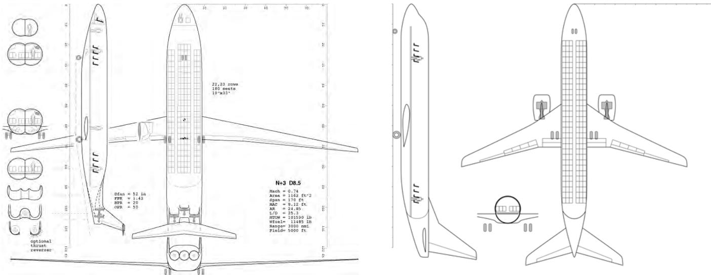
The D Series aircraft fuselage (left) is shorter and wider than that of a 737 (right). It provides three times the percentage of the overall lift on the aircraft, compared to that of the 737 fuselage (approximately 6 percent for 737).
