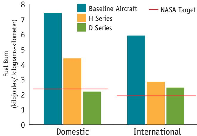
Performance of the D and H series aircraft compared with NASA N+3 targets
