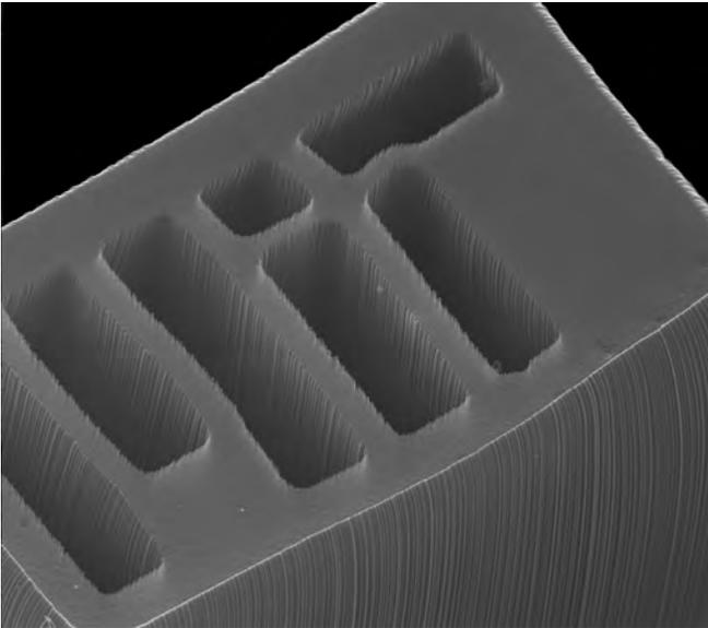
Aligned carbon nanotubes are organized as an MIT logo via photolithography and then grown in Wardle’s lab. The aligned CNT “forest” appears optically and under scanning electron microscopy (as in the image) as black and solid, however, it is more than 99 percent air by volume. Aligned CNT forests like this are used in Wardle’s energy storage and composite research.
