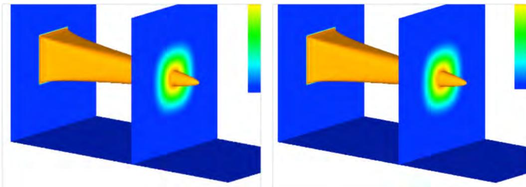
Reduced-order models are essential for reducing the computational time of reacting flow simulations for use in design and control applications. Here, a finite element model takes 13 hours CPU time to estimate the fuel concentration for a jet diffusion flame in a combustor (left). The reduced-order model (right) solves the same problem in a few seconds with high levels of accuracy. (D. Galbally, K. Fidkowski, K. Willcox, O. Ghattas image)
