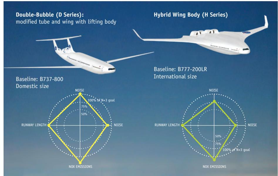
Rendering and performance assessment of two MIT aircraft designs relative to the four N+3 NASA targets. The circles on the small graphs represent the 50 percent, 75 percent and 100 percent target levels targets, and the solid symbols indicate the performance of the concept aircraft.
