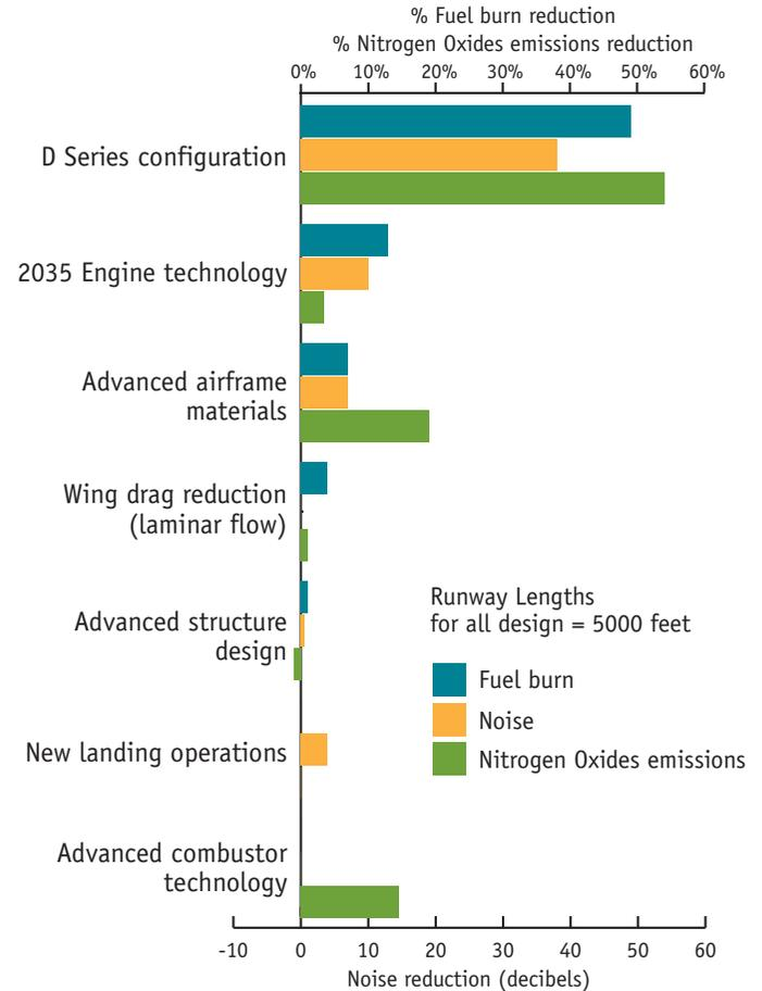
The D series configuration offers major performance benefits even with current technology. This chart shows the effect of configuration change on the NASA targets (the top three bars) compared with the benefits brought by changes in technology (the bars in all the other categories).
