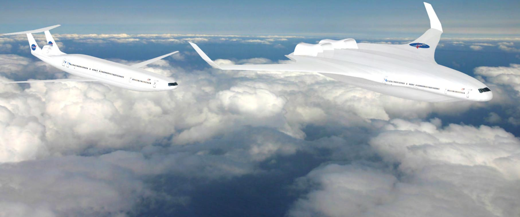
MIT's designs for two future aircraft: the D Series (left), a double-bubble configuration, which is a 180-passenger plane, and the H Series, a blended-wing body which is a larger 350-passenger plane. Both would offer major fuel, noise, engine emissions, and runway length reductions compared to aircraft of today. (MIT/Aurora Flight Sciences image)
