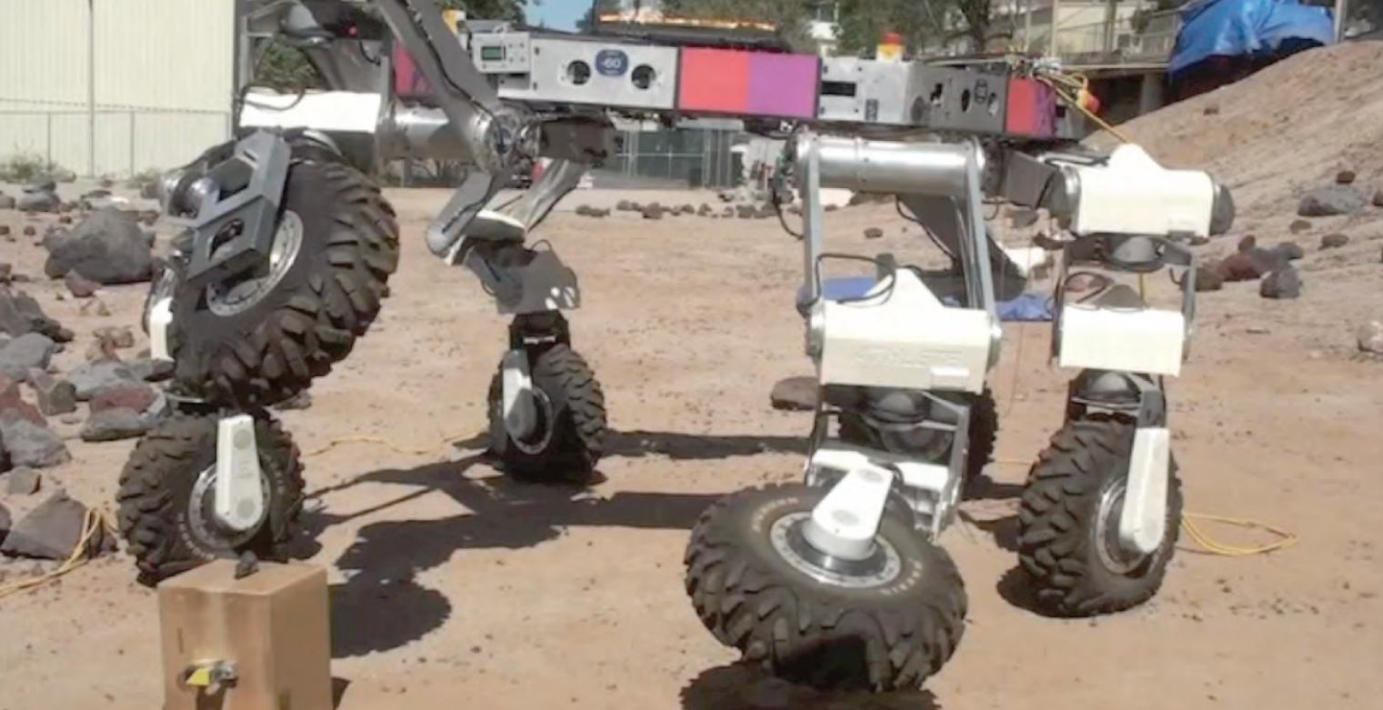
The Model-based Embedded and Robotic Systems group has developed methods for controlling walking machines and applied them to such vehicles as such as the NASA Jet Propulsion Lab's Athlete robot, a six-legged/wheeled lunar rover that performs heavy lifting and manipulation tasks by using its legs as arms.
