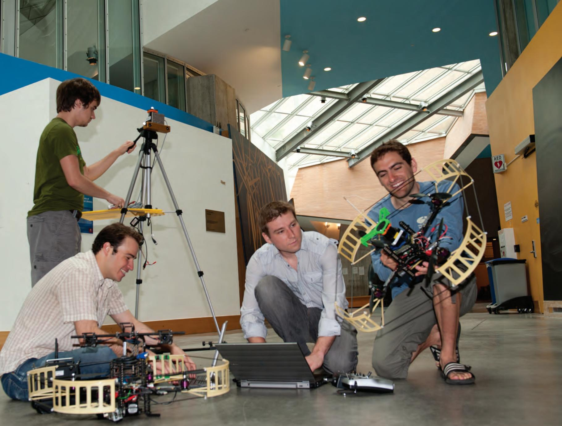
Students (from left) James Wiken (standing), Abraham Bachrach, Samuel Prentice, and Adam Bry prep a pair of quadrotor helicopters to fly through MIT's Stata Center, exploring and mapping the building. Equipped with a variety of sensors for operating in different environments, the rotorcraft can fly in complex, populated environments. (William Litant/MIT photo)
