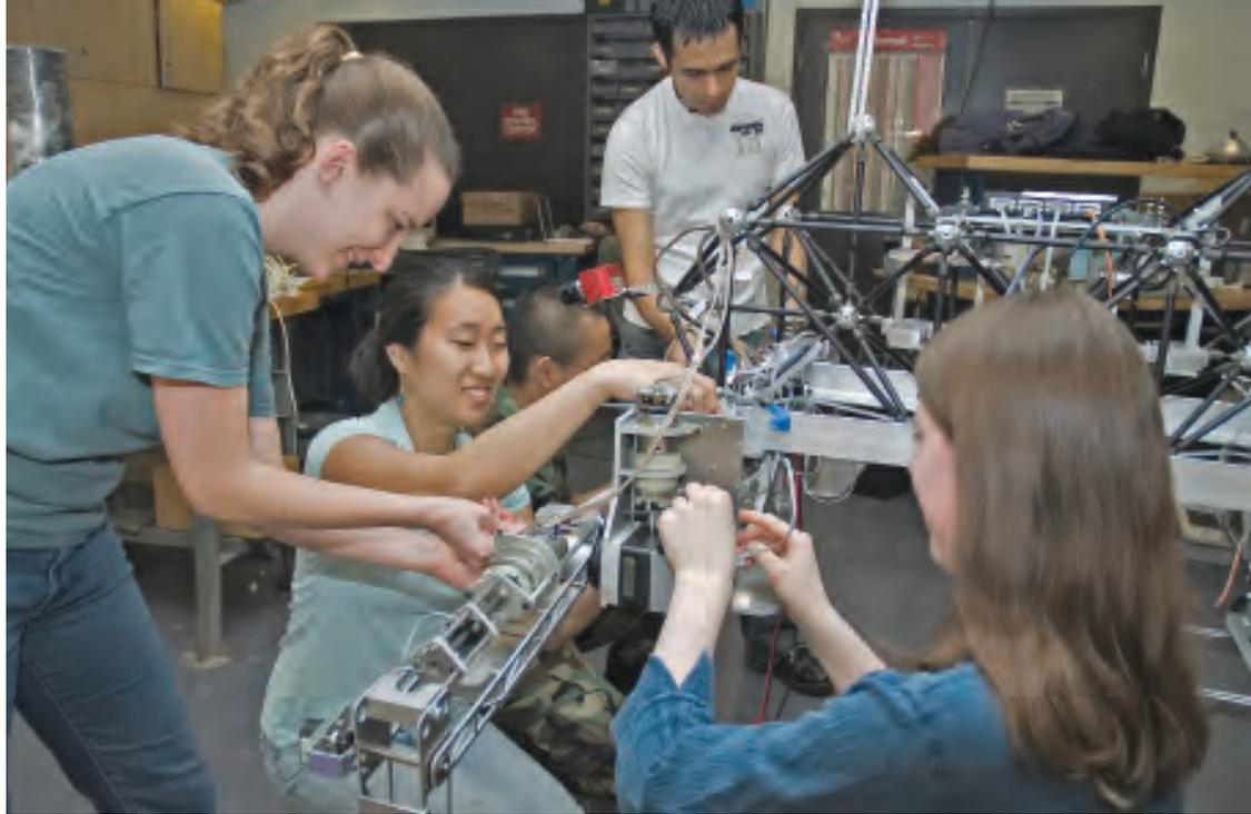
AeroAstro capstone course students assemble Moretta, a legged planetary rover they designed and built to traverse terrain that would stymie a wheeled vehicle. (William Litant/MIT photo)
