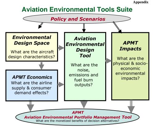
Figure 2.1 Modelling Blocks within the Aviation Environmental Tools Suite
