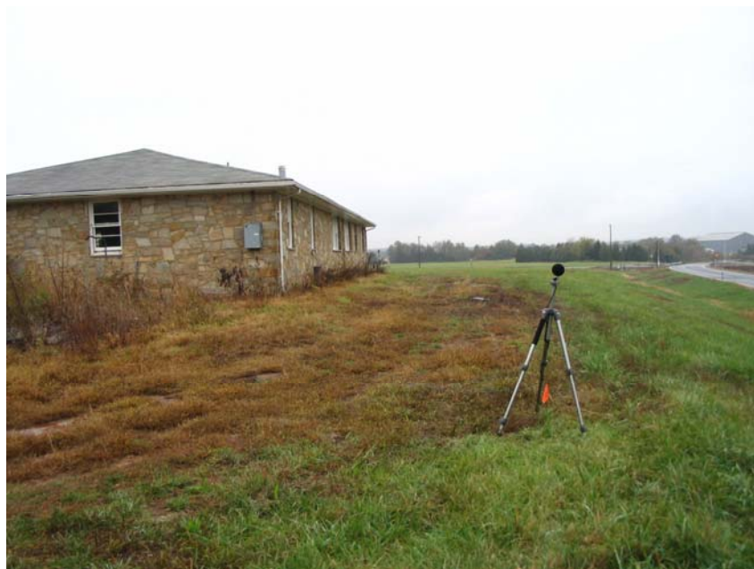
Figure 10. Exterior view of Stone House looking from the east. Runway 30 is approximately 3100 ft (960 m) to the west (towards the background). One of the outdoor microphones is shown in the foreground.
