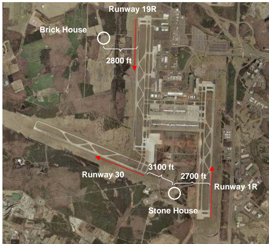
Figure 5. Overhead photograph of Washington Dulles International Airport (IAD) showing the runway layout, locations of the residential structures and their proximity to the runways. The arrows indicate the predominant direction of runway traffic during the measurements. (Image courtesy of the USGS.)
