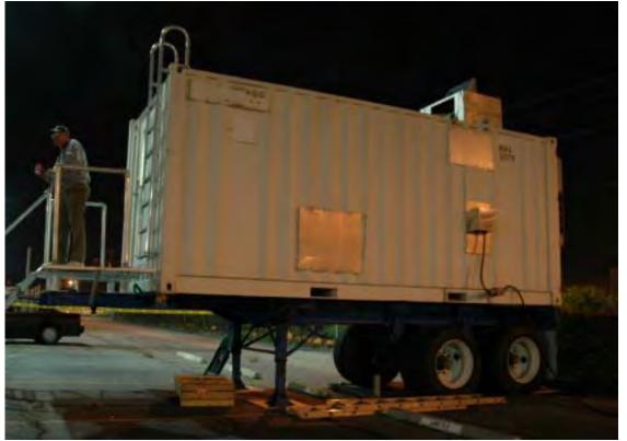
Figure 2: LIDAR system for plume geometry and emission rate measurements. The enclosure on top contained the elevation-scanning mirror.
