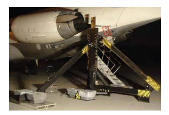
Figure 1: Probe stand used to sample jet exhaust
