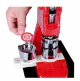
Place metal badge top (rim down) in left hand die in circular slot. Cover with cut out print (printed side up) and one plastic film.
