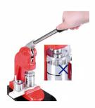
Place pinned back (zigzag side of pin showing) in right hand die. Press down the handle to complete assembly. There must be no gap in the top die when you press down the handle.
