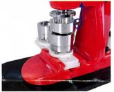
Align die set into the body groove.
