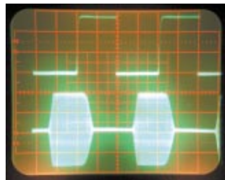
Figure 3—CW keying waveform for the 6N2 showing the first two dits using external keying. Equivalent keying speed is 60 WPM. The upper trace is the actual key closure; the lower trace is the RF envelope. The transceiver was being operated at 20 W output at 144.02 MHz.
