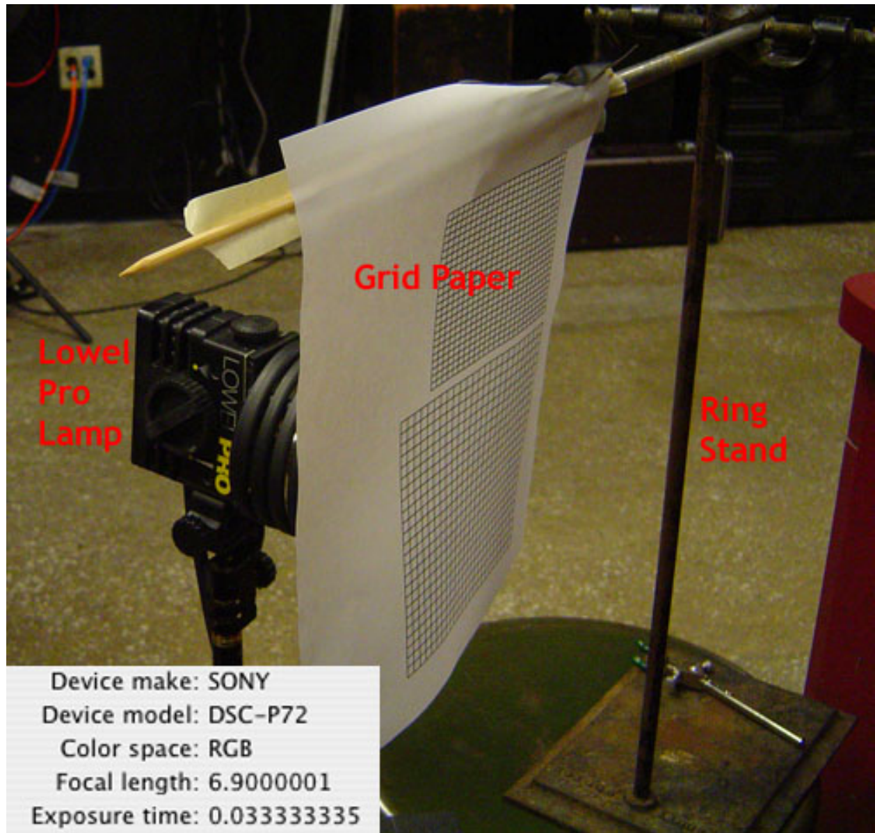
Figure 11: A figure of the method used to project the grid onto the glass for this high-speed camera setup. The grid paper is formed by printing a grid onto paper. The paper is held by taping it to a ring stand.
