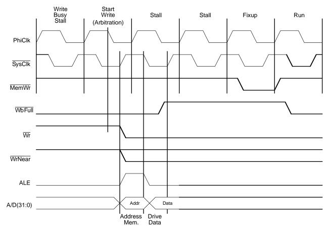
Figure 9.5. Write Buffer Full Operation
