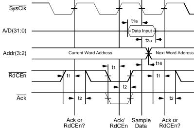
Figure 8.4. Data Sampling on the R3041
