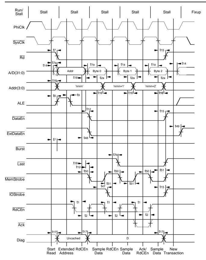
Figure 8.23. Tri-Byte Read Without Bus Wait Cycles
