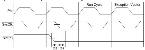
Figure 6.6. Synchronized Interrupt Operation
