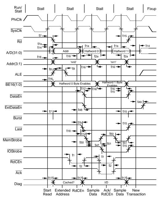
Figure 8.18. Mini-Burst Halfword Read Without Bus Wait Cycles
