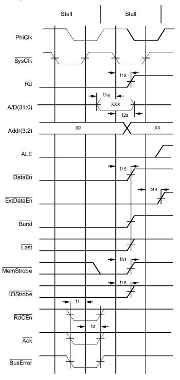
Figure 8.15. Block Read Terminated by Bus Error
