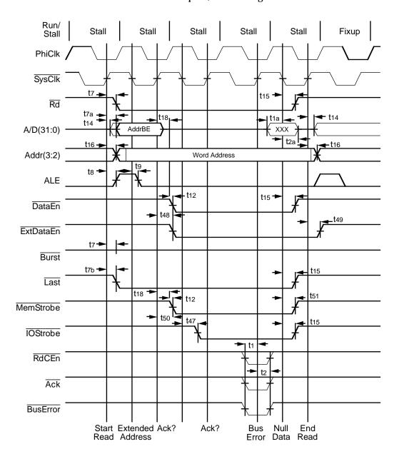
Figure 8.14. Single Word Read Terminated by Bus Error
