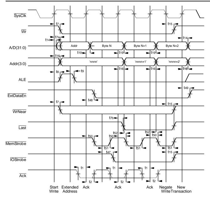
Figure 9.16. Three Byte Mini-Burst 8-Bit Port Write
