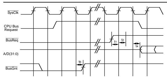
Figure 10.4. DMA Protocol BusGnt De-assertion
