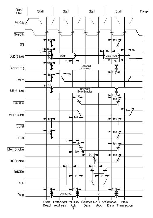
Figure 8.17. Single Halfword Read With Bus Wait Cycle
