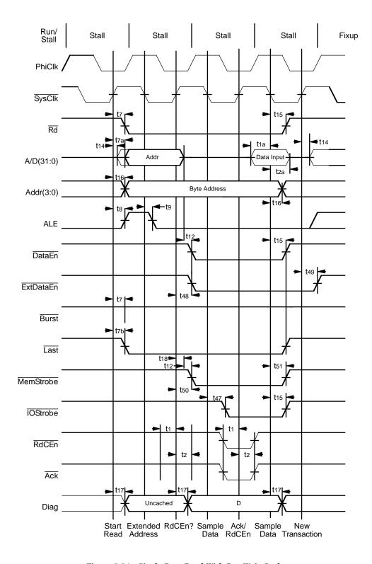
Figure 8.21. Single Byte Read With Bus Wait Cycles
