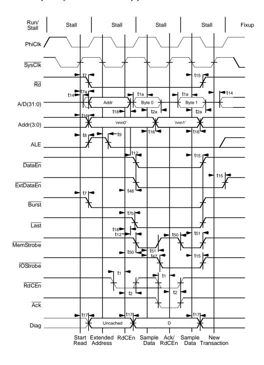
Figure 8.22. Double Byte Read Without Bus Wait Cycles
