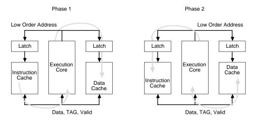
Figure 3.3. Phased Access of Instruction and Data Caches
