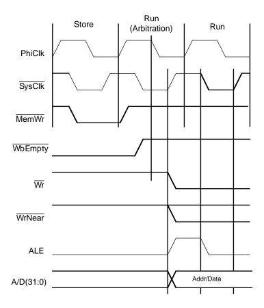
Figure 9.1. Start of Write Operation - BIU Arbitration
