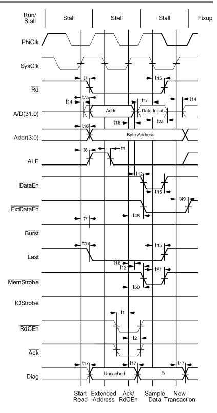
Figure 8.20. Single Byte Read Without Bus Wait Cycles
