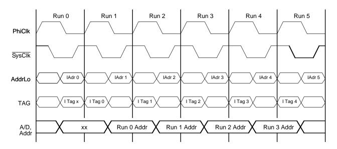
Figure 12.1. R3041 Debug Mode Instruction Address Display
