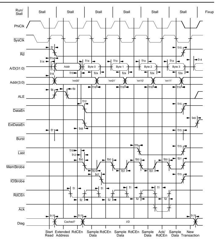
Figure 8.24. Quad-Byte Read Without Bus Wait Cycles
