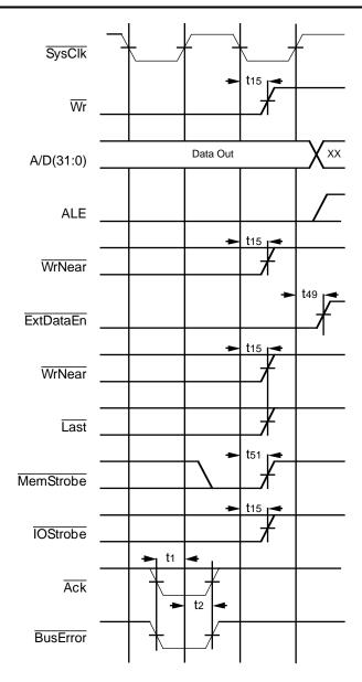
Figure 9.12. 16-Bit Write Terminated by Bus Error
