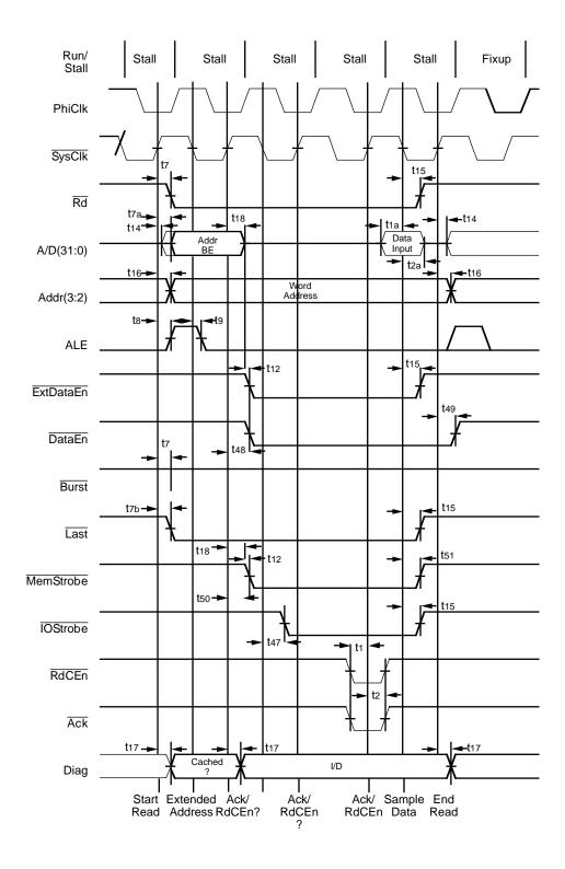
Figure 8.10. Single Word Read With Bus Wait Cycles
