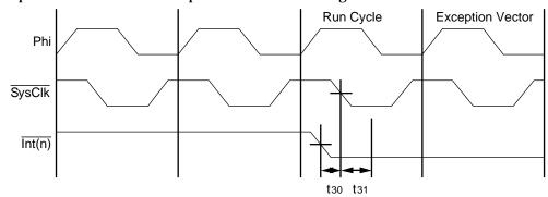
Figure 6.7. Direct Interrupt Operation
