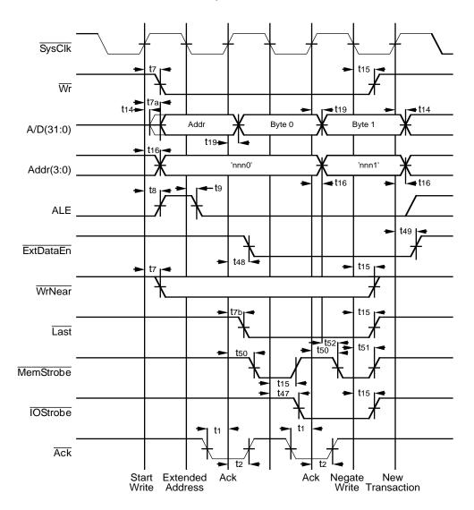
Figure 9.15. Two Byte 8-Bit Port Write with Wait Cycles
