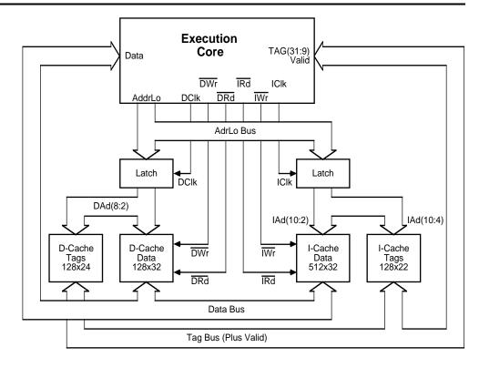
Figure 3.2. R3041 Execution Core and Cache Interface
