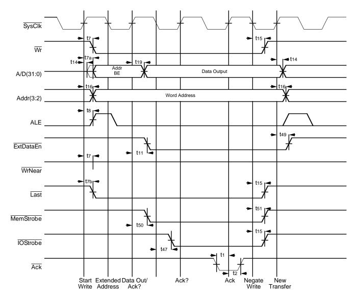
Figure 9.7. Basic 32-Bit Port Write with Wait Cycles
