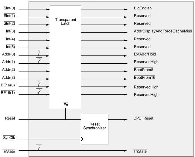
Figure 11.4. Configuration Mode Initialization Logic
