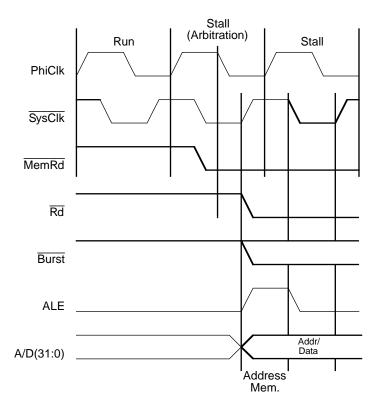
Figure 8.1. CPU Latency to Start of Read
