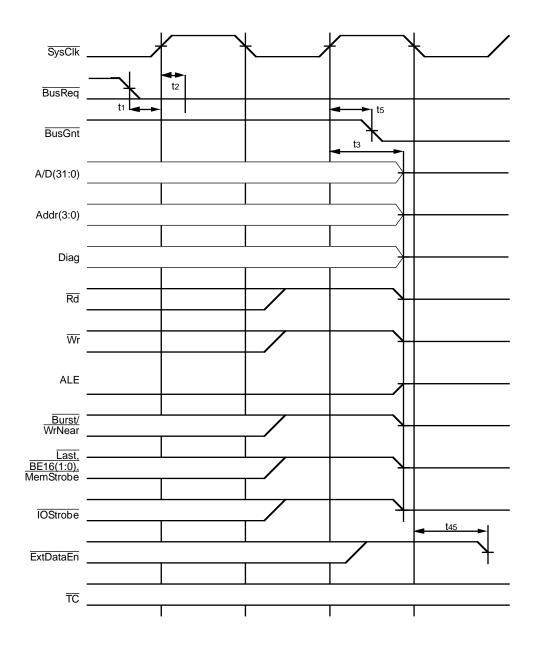
Figure 10.2. Bus Grant and Start of DMA Transaction
