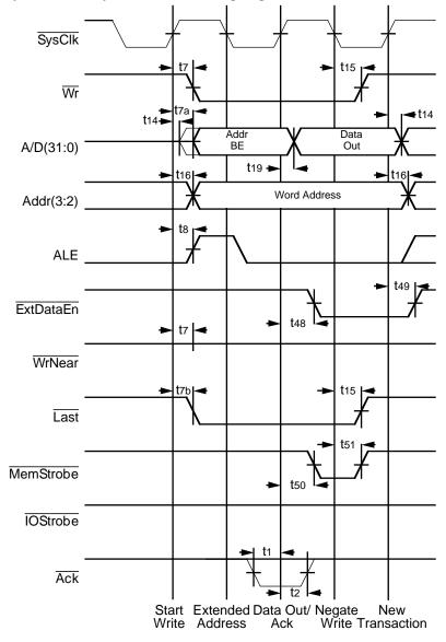
Figure 9.6. Basic 32-Bit Port Write with No Wait Cycles
