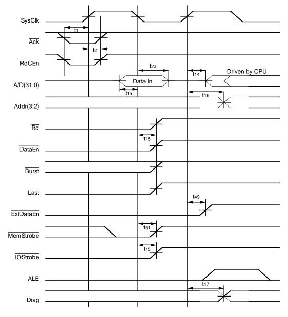
Figure 8.5. Read Cycle Termination
