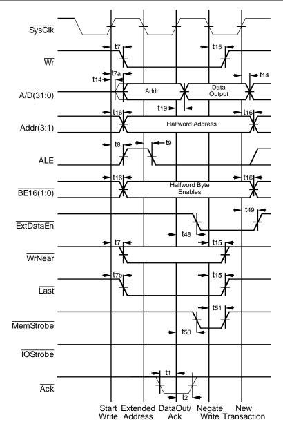
Figure 9.9. Single Datum 16-Bit Port Write with No Wait Cycles
