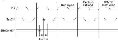
Figure 6.8. Synchronized BrCond Inputs
