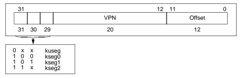
Figure 4.1. Virtual Address Format
