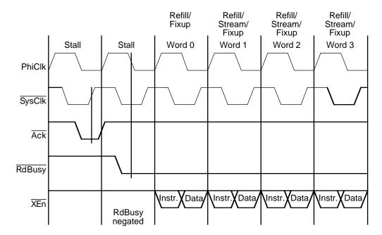
Figure 8.7. Internal Processor States on Burst Read
