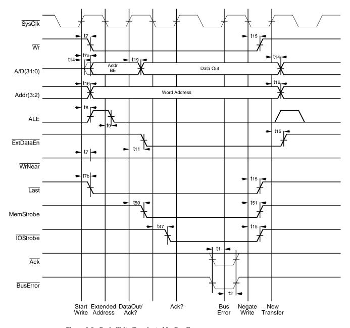
Figure 9.8. Basic Write Terminated by Bus Error
