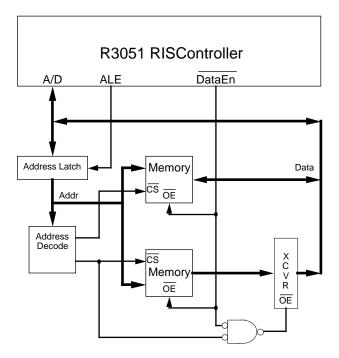
Figure 8.6. Use of DataEn as Output Enable Control
