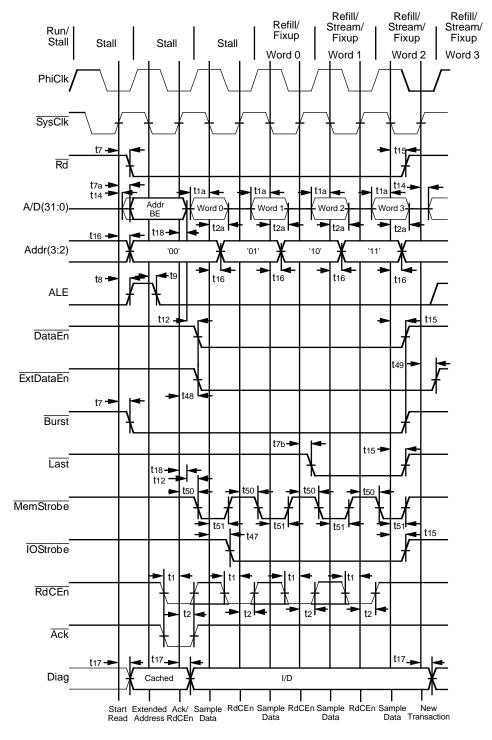
Figure 8.11. Burst Read With No Wait Cycles
