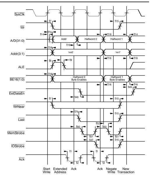
Figure 9.11. Mini-Burst 16-Bit Port Write
