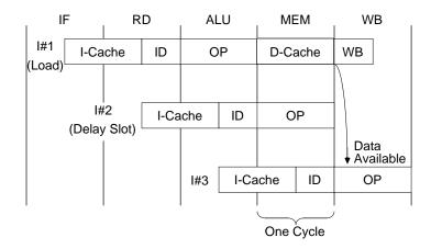
Figure 2.7. Load Delay
