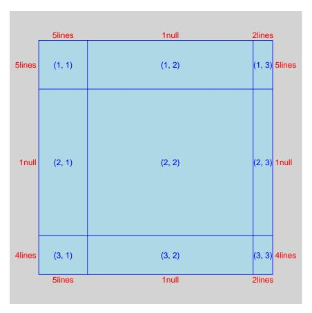
Next we create a set of viewports which will occupy different areas within the layout, corresponding to the margins for axes and labels, and the plotting region.
