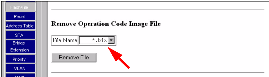
Figure 25: Removing an operation code image file
