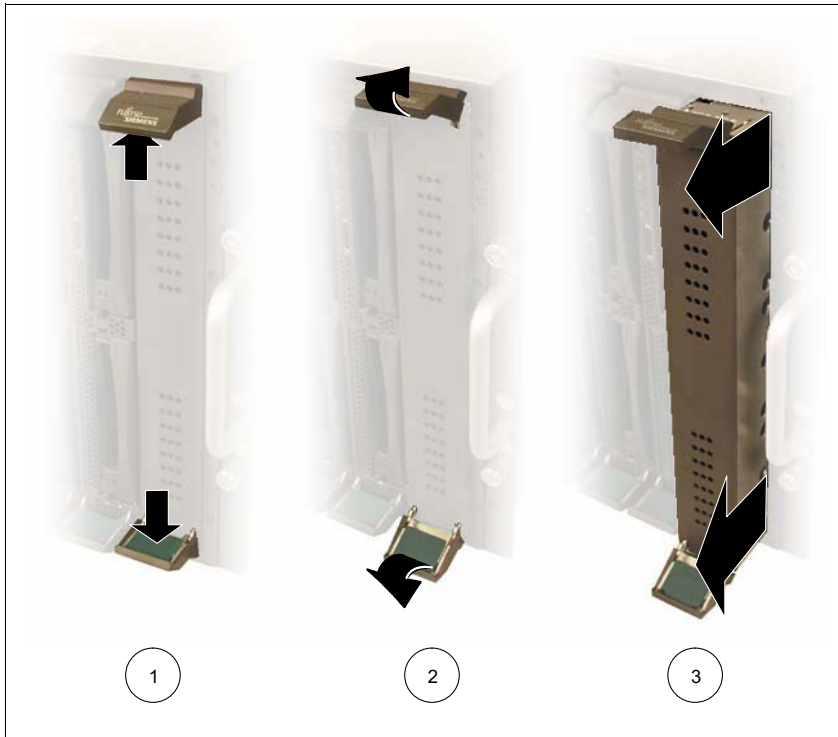
Figure 5: Removing the dummy module for a server blade
