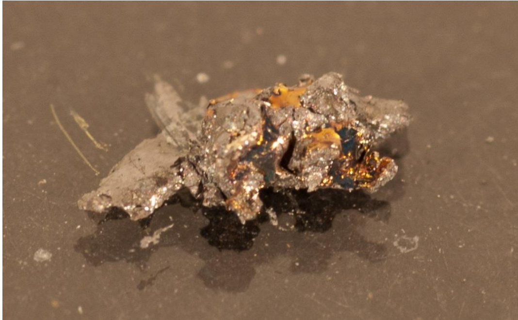
Close up of solidified bismuth. Color variation from crystal formation is visible. Size is roughly ~3 mm across. f/16, 90mm lens
