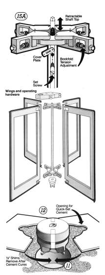
16B. Install the center shaft by setting the base of the shaft into the floor pivot. Align the shaft with the speed control and reseat the control and replace the 8 mounting screws.
