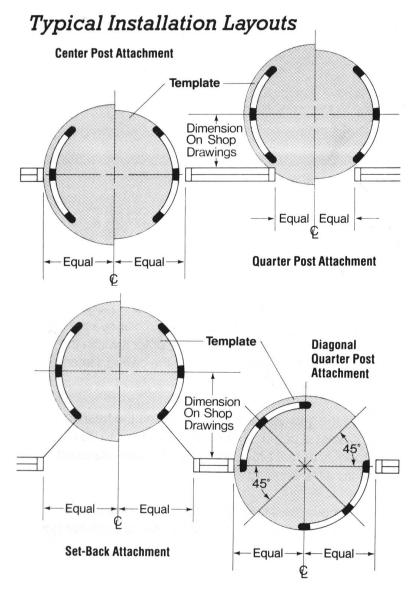
**4.** Drill pilot holes in the floor at the center and for all anchors. Drill all anchor holes: 1/2" diameter x 2 1/2" deep.
