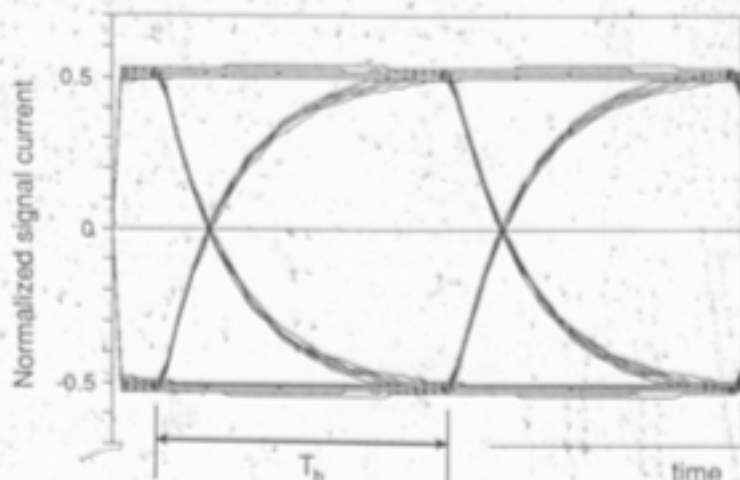
Figure 3.10 Signal eye diagram for a first order LPF with bit rate, R , equal to the filter noise equivalent bandwidth, B .
