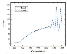
Fig. 2. (Color online) Spectral group delay of an example chirped mirror. A portion of the response past the high reflectivity region (wavelengths greater than approximately 1050 nm) is shown to demonstrate that the approximation holds even when the group delay is rapidly varying.
