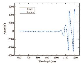
Fig. 3. (Color online) Spectral group delay dispersion of the chirped mirror shown in Fig. 2.
