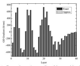
Fig. 4. Exact and approximate gradient of the group delay of the filter shown in Fig. 2 at 800 nm. The gradient approaches zero for layers past the 40th as virtually all of the light is reflected by that point.
