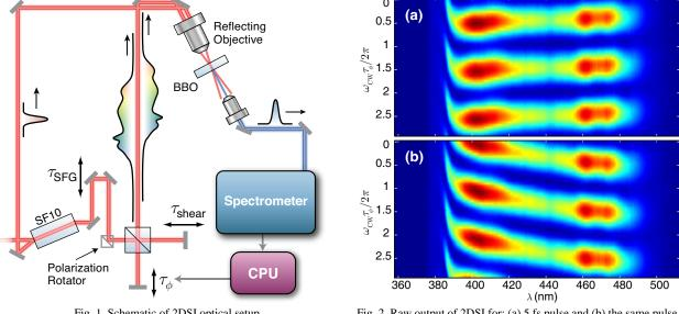
Fig. 1. Schematic of 2DSI optical setup.
