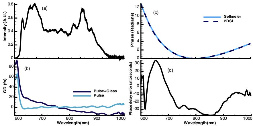
**Fig. 3.** Few-cycle pulse characterization: (a) spectrum of pulse; (b) spectral group delay of pulse before and after dispersion by glass plate; (c) extracted phase difference (dashed) and theoretical (solid) prediction for fused silica; (d) phase delay error computed from (c).
