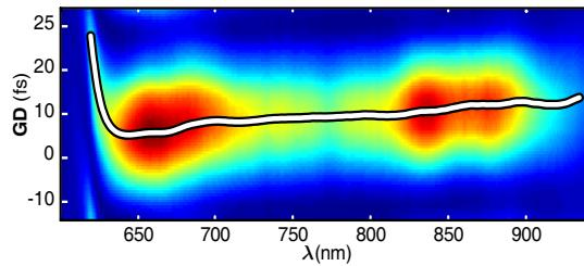
**Fig. 2.** A single 2DSI fringe from a 5 fs Ti:sapphire pulse, with the extracted spectral group delay superimposed, demonstrating the simple interpretation of the fringes.
