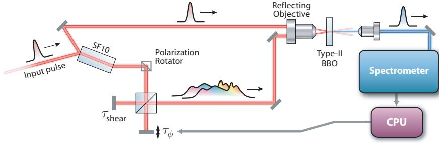
**Fig. 1.** Schematic of 2DSI optics.
