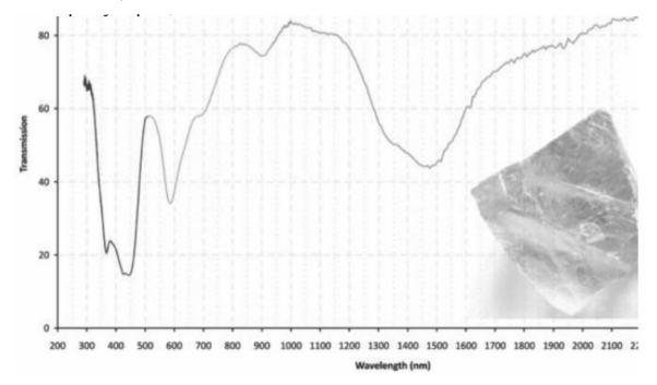
**1.8** The figure below shows the absorption spectrum of the colorless mineral **X** after its treatment with gamma rays. Determine the color of the mineral.
