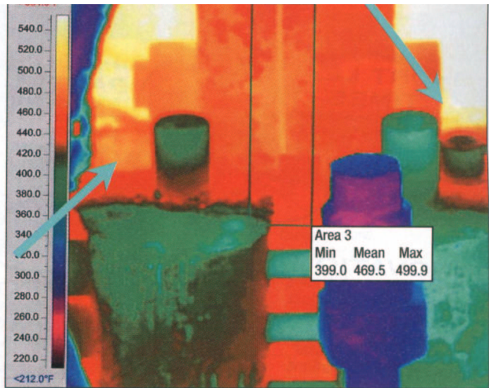
Fig. 7. The arrows point to the areas where the bolts would be replaced.
