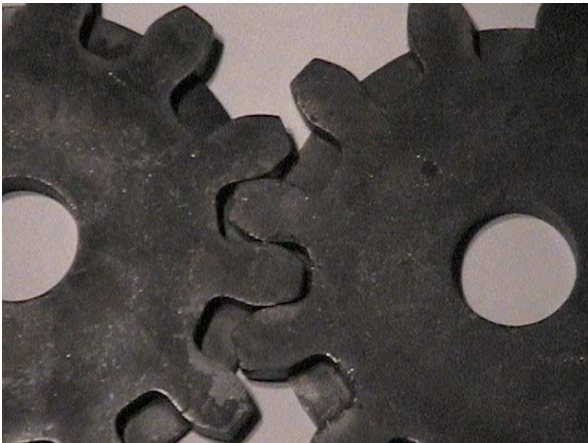
Figure 2-1 Gear teeth meshing.
