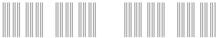
Fig. 7. The priority data bits are used to refine a point on a Cantor set. The natural tree structure of the Cantor set construction allows us to encode bits sequentially. The Cantor set also has finite gaps between all points corresponding to bit sequences that first differ in a particular bit position. These gaps allow us to reliably extract bit values from noisy observations of the Cantor set point regardless of which point it is.
